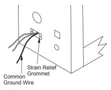
Figure 12 - Wiring Through Outer Surround
